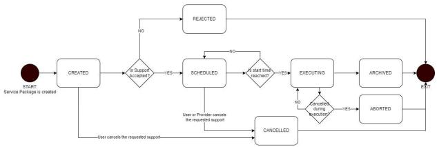
Fig. 4. Service Package Status State Machine in GSSNG
