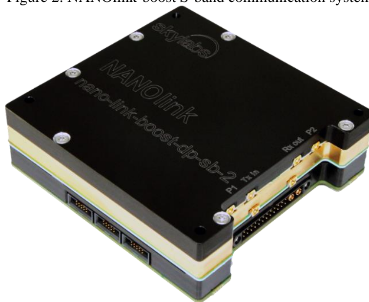
Figure 3: NANOLink-boost-dp S-band communication system with diplexer
