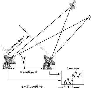
To enable a delta-DOR measurement, a spacecraft must emit several tones. The characteristics of the tones are selected based on the requirements for phase ambiguity resolution, measurement accuracy, efficient use of spacecraft signal power, efficient use of ground tracking resources and the frequency allocation for deep space tracking.
