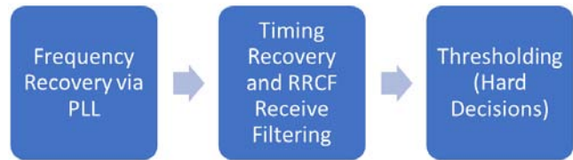
Figure 6: Software-receiver architecture for demodulation of recorded Iris output.
