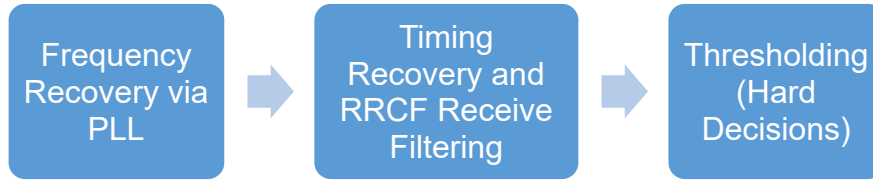
Figure 21. Software-receiver architecture for demodulation of recorded Iris output.
