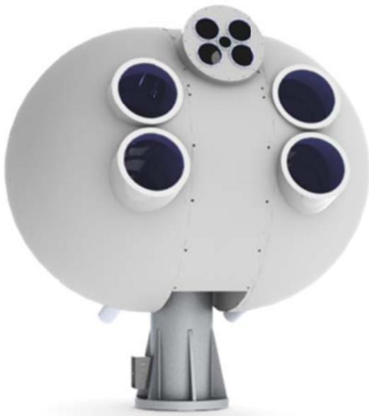
Figure 75: Lunar Lasercom Ground Terminal will be enhanced with Adaptive Optics and a DPSK Modem.
