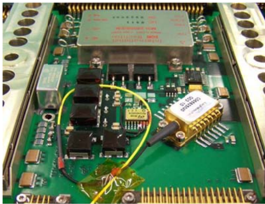
Figure 15: Space-qualified directly modulated laser diode.
