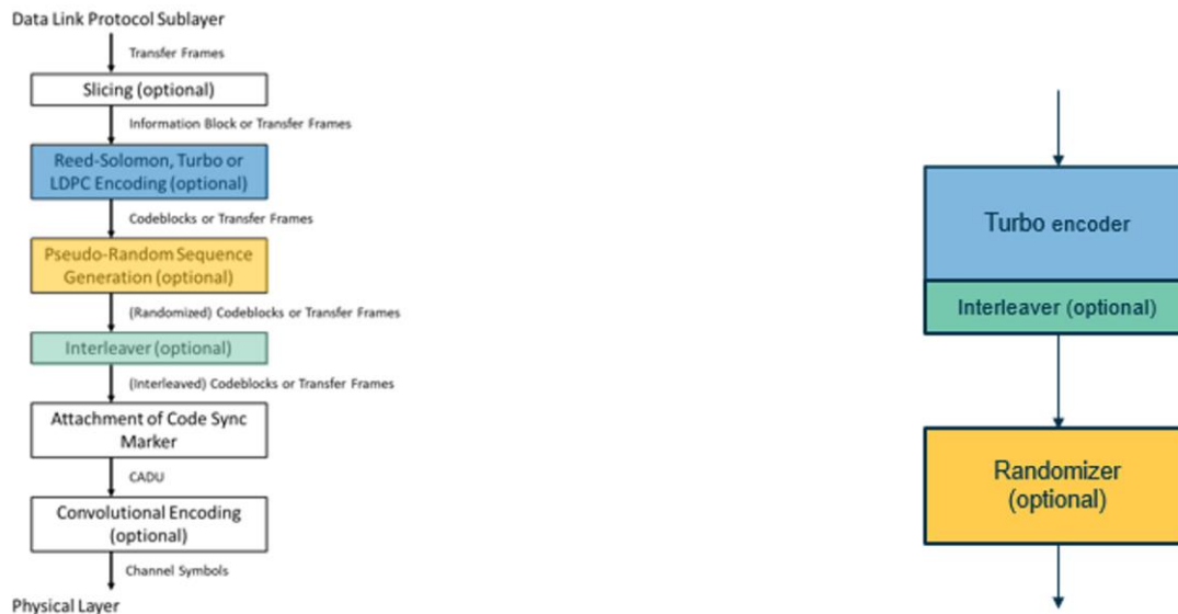
Figure 1: comparison of the eventual 131.0-B functions if Turbo channel interleaver is placed after pseudo-randomizer (left) vs being placed before (right).
