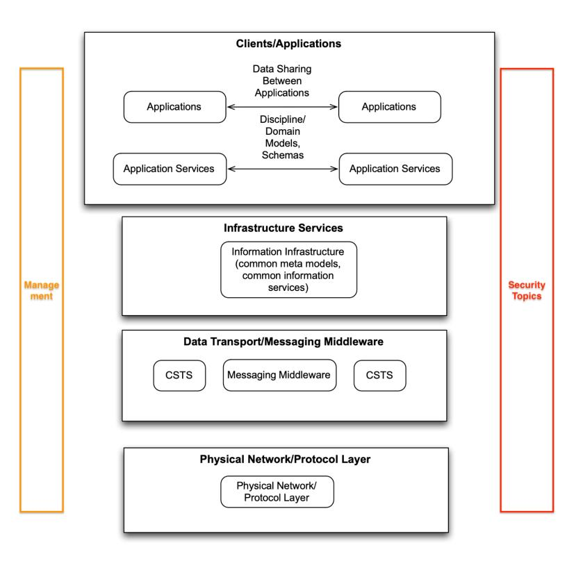
Figure 4-6: Information Service View of the CCSDS Layered Stack
