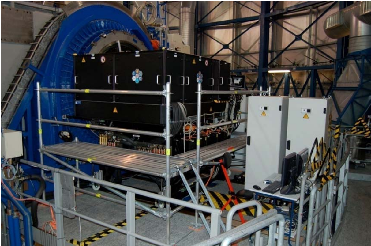
Figure 1 APE fully installed on Melipal Nasmyth A.
