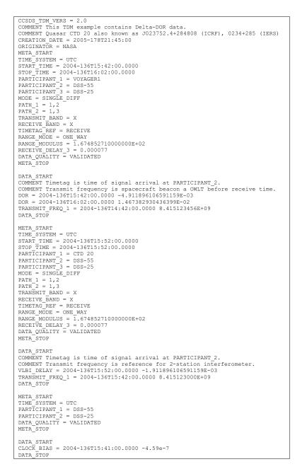
Figure E-11: TDM Example: Delta-DOR Observable
