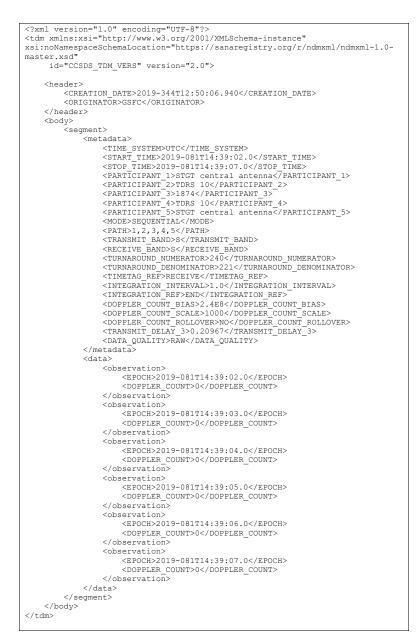
Figure E-24: TDM Example: Use of Doppler Counts
