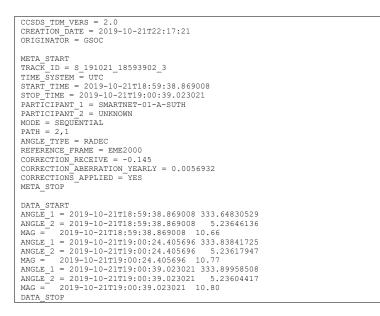
Figure E-23: TDM Example: Use of 'TRACK\_ID'
