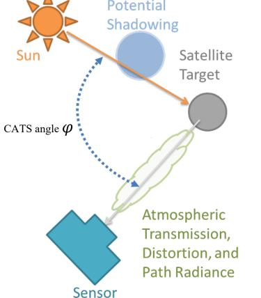
Fig. C- 2 Depiction of optical viewing Critical Angle to the Sun (CATS) angle geometry
