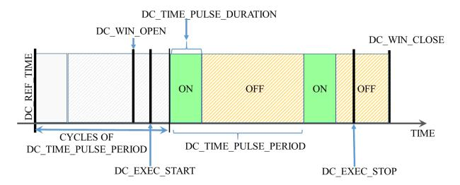
Fig. C- 3 Diagram of time-based duty cycle (DC TYPE = "TIME")
