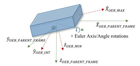
Fig. C- 1 Depiction of Optimally-Enclosing Box and definitions of MAX, INT, and MIN orientation vectors relative to OEB parent frame
