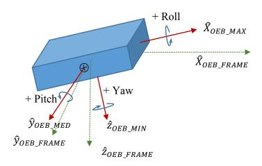
A fixed orientation of the OEB with respect to the user-specified "OEB\_FRAME" is defined using an ordered sequence of Euler rotations that map from the user-specified OEB\_FRAME to the Optimally-Encompassing Box vector directions. The above figure shows the proper definitions and adopted sign conventions for Yaw, Pitch and Roll angles. The resulting transformation sequence is:
