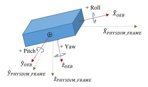
A fixed orientation of the OEB with respect to the user-specified "PHYSDIM\_FRAME" is defined using an ordered sequence of Euler rotations that map the OEB frame into the PHYSDIM\_FRAME. The above figure shows the proper definitions and adopted sign conventions for Yaw, Pitch and Roll angles. The resulting transformation sequence is:
