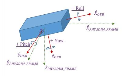
A fixed orientation of the OEB with respect to the user-specified "PHYSDIM\_FRAME" is defined using an ordered sequence of Euler rotations that map the OEB frame into the PHYSDIM\_FRAME. The above figure shows the proper definitions and adopted sign conventions for Yaw, Pitch and Roll angles. The resulting transformation sequence is:
