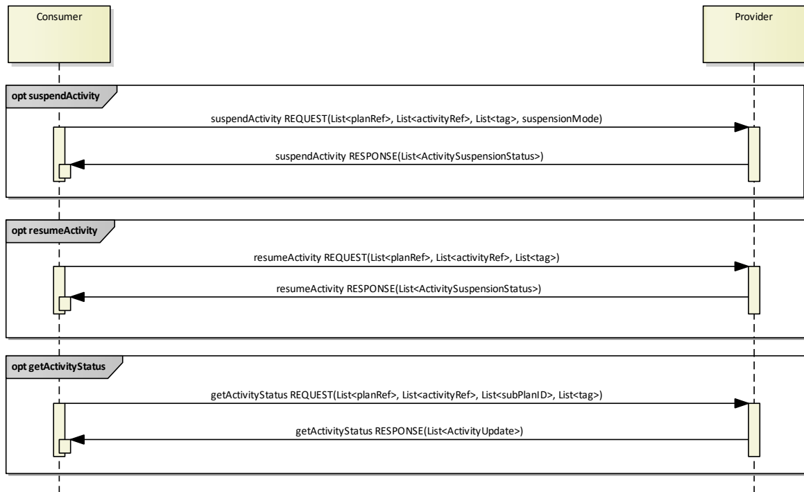
Figure 3-9: Activity Execution Control Operations
