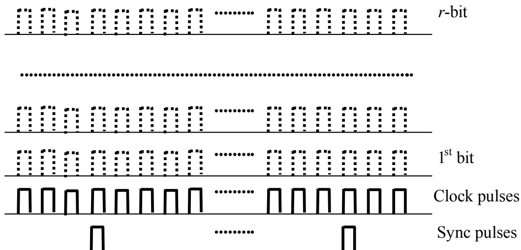
Figure 3-1: Graphs of Signal (Structure of Data) at the Diverse Channel Output (Software-Hardware Output For Correlated Data Generation)
