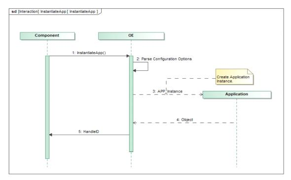
Figure 11: Sequence Diagram for InstantiateApp
