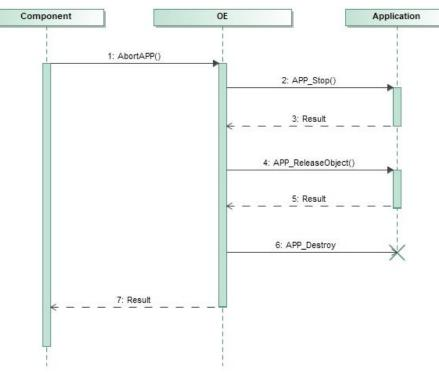
Figure 12: Sequence Diagram for AbortApp
