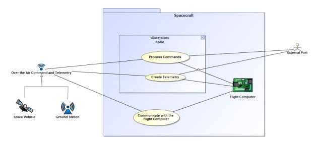
Figure 16: Command and Telemetry Interfaces
