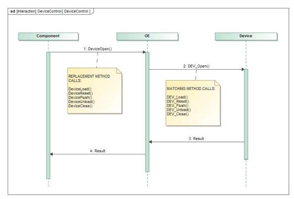
Figure 13: Sequence Diagram for Device Control Component
