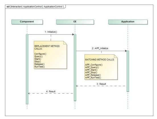
Figure 10: Sequence Diagram for Application Control Component
